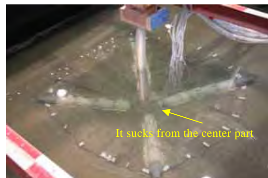
Fig.15 Situation of the sediment discharge (The bottom of all length of the pipe is cut)
