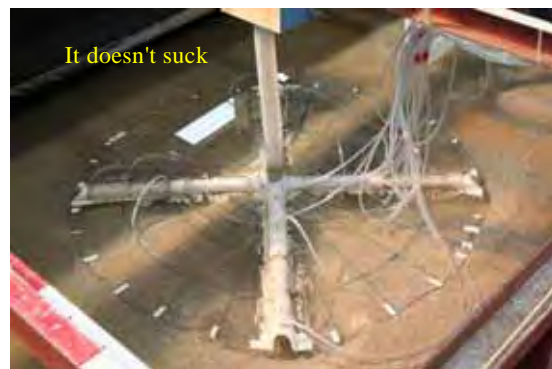
Fig.16 Situation of the sediment discharge (Bottom cut parts are installed at the edge)
