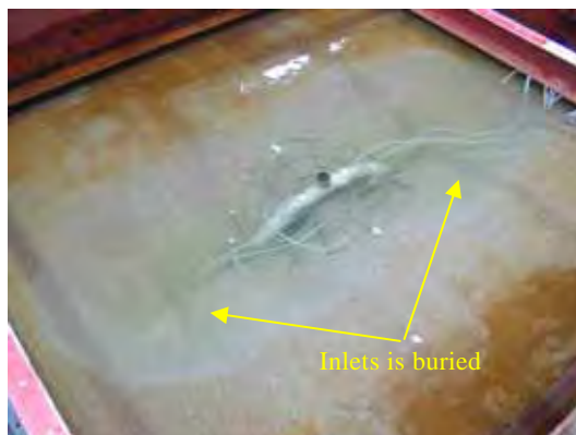
Fig.13 Situation of the sediment discharge (Two inlet layout)
