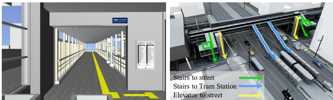
Figure 9. Station exit and Entrance in the newly-established pedestrian bridge
