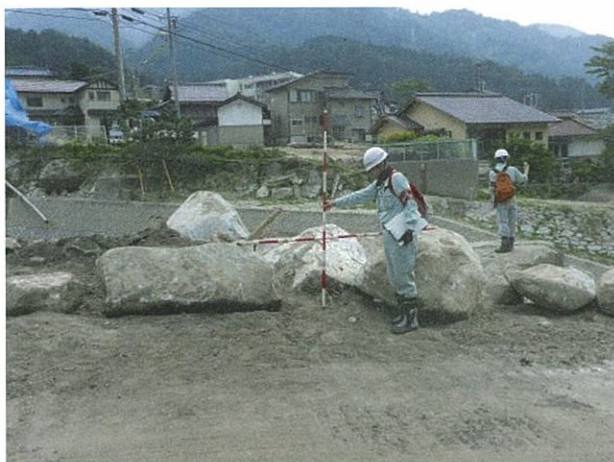
写真-15 氾濫域（梨子沢右岸）での巨礫の堆積状況 Photo 15 Large boulder deposited on right bank of Nashizawa river
