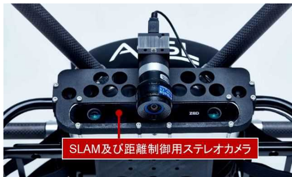
Fig. 3 Stereo camera for SLAM and distance control
