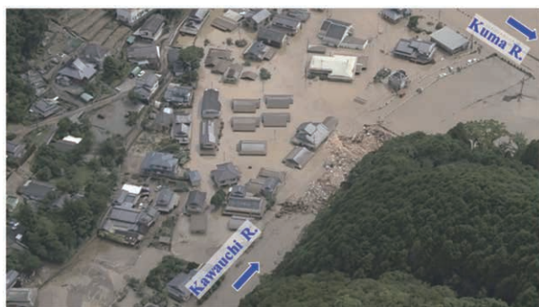
Fig.23 Flood retention in the Kawauchi River due to backwater effect from the Kuma River (photo taken on July 4, 2020, courtesy of Kyushu Regional Development Bureau, Ministry of Land, Infrastructure, and Transport)
