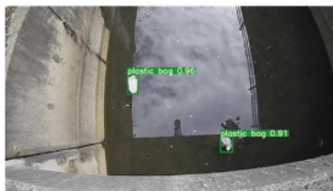
Figure 8 Example of artificial debris discrimination in the drainage channel in Case3 with the dataset-C. (Photo taken at 10:20, March 2, 2020)
