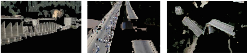
Fig. 8. Bridge collapse and interruption color segmentation K-means clustering results.
