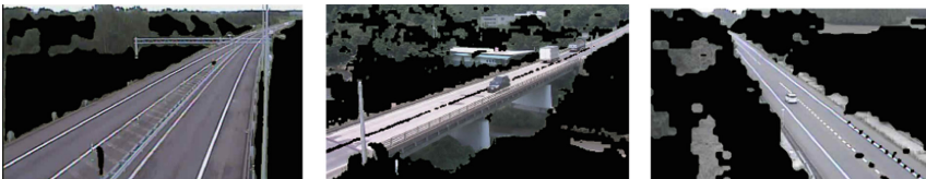
Fig. 6. Infrastructure color segmentation K-means clustering results.
