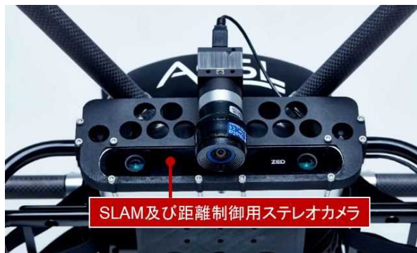
Fig. 3 Stereo camera for SLAM and distance control
